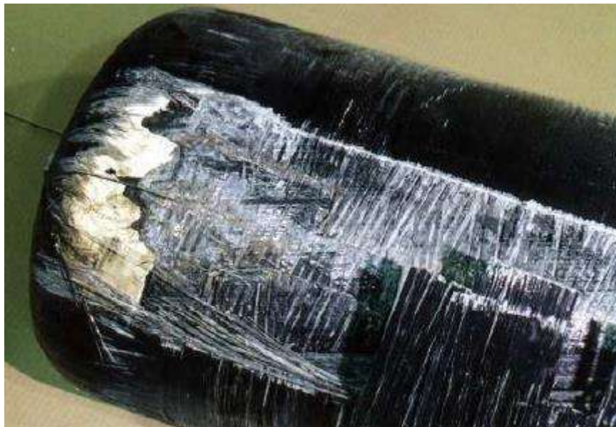
Fig.23.: Bus tank after impacted with an over-bridge [28]
