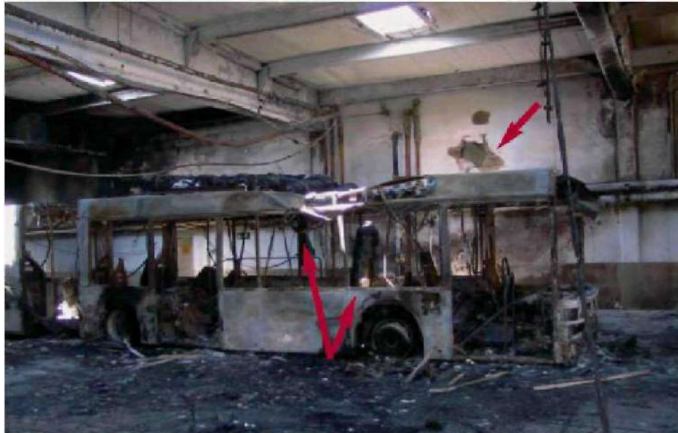
Fig.26.: The above arrow shows where the wall was leaked through by the exploded tank [24]
