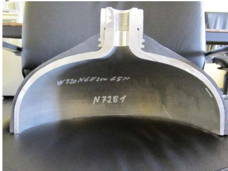
Fig.12.: Type 3 vessel cross section at the neck part [photo: Dynatek]
