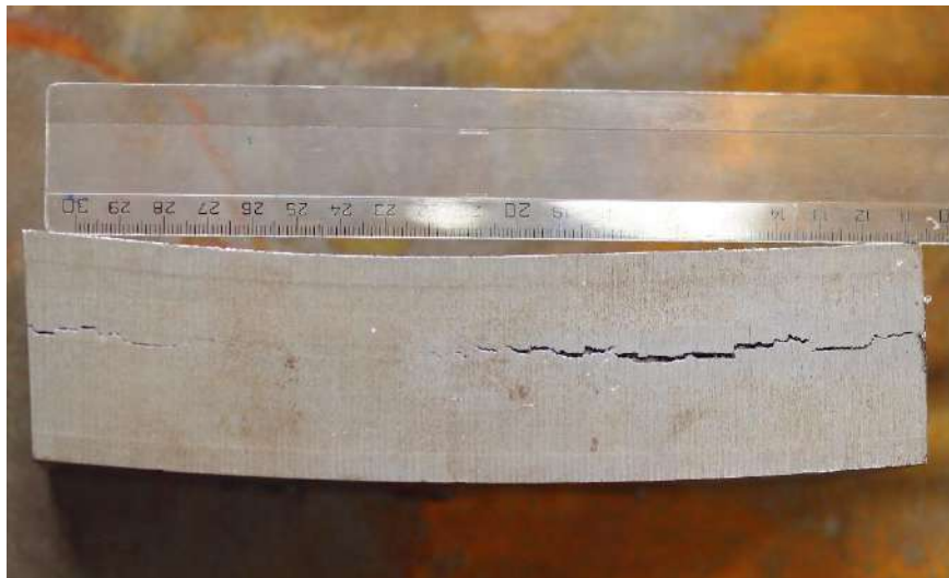
Fig.4.: This excised piece of a hydrogen industrial spherical container shows the hydrogen accumulation deep in the 50 mm wide steel plate, which was even able to straighten the inner side. Under heat and pressure the Hydrogen bubble created bursting force is over 100 MPa range. [Author]
