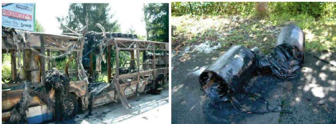
Fig.27.: The burned out bus in Montbéliard, and the residue of the cylinder, which splitted in two parts. The initial problem came from the electrical circle of the bus [24]
