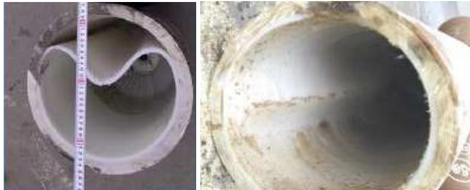
Fig.22.: The blistered liner can see on the left cut up cylinder, at low pressure the strung-out liner come off the epoxy-fibre layer, and the hydrogen accumulating between. On the right the one already cracked liner is visible. The increase of the hydrogen passage through the wrapping resulted. [Source of the photo is uncertain]
