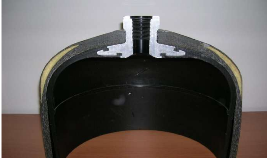
Fig.13.: Type 4 vessel cross section at the neck part [photo Dynatek]
